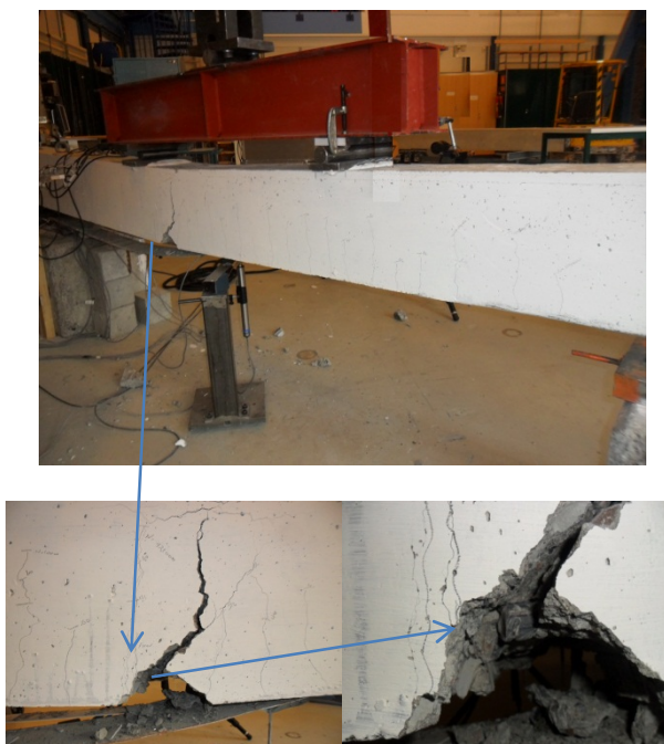
(c) Plate strengthened beam (B1-EE1-F)
